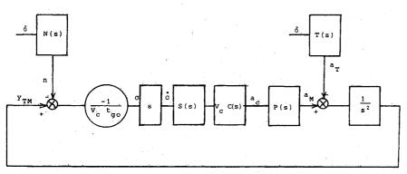
Fig. 2 Angular guidance loop.
